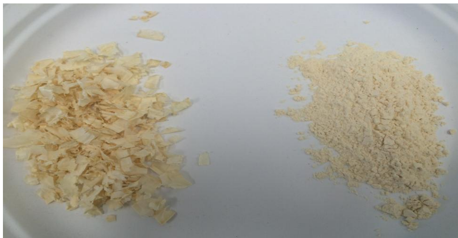
Figure 18: Raw sawdust (left) and sawdust powder ( <116 \mu\text{m} ).
