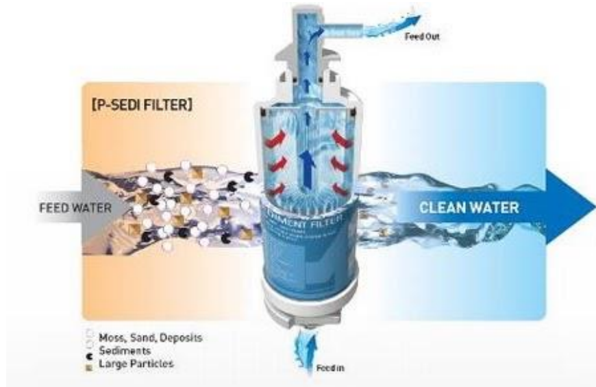
Figure 35. A microfiltration system filtering out sediments and solid particles for clean drinking water.
