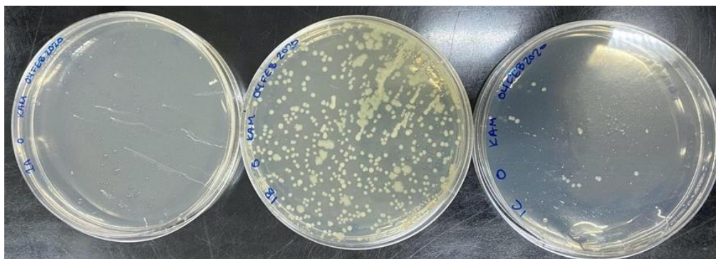
Figure 22. From left to right: Source, pre-filter and point of use bacterial contamination at the Bamrung 87 school. All plates non-diluted, 100 \mu L water sample incubated at 36°C for 24 hours.
