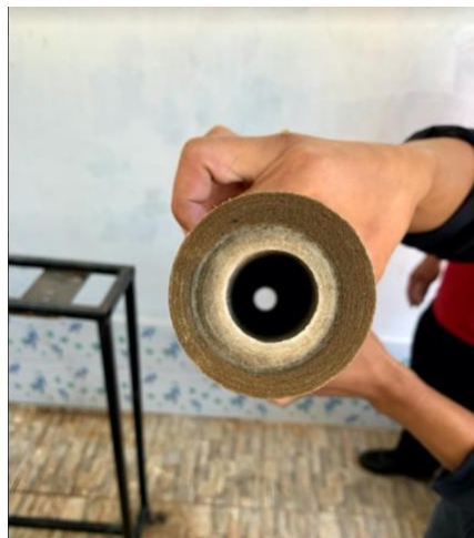
Figure 24. Microfilter membrane at Bamrung 87 school after three months.
