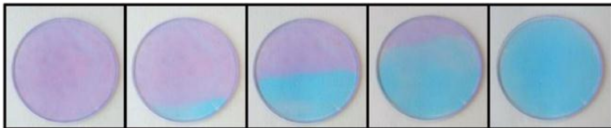
Figure 2-2. Photographs of MB/urea/HEC humidity indicator during color change after exposure to 100% relative humidity 2
