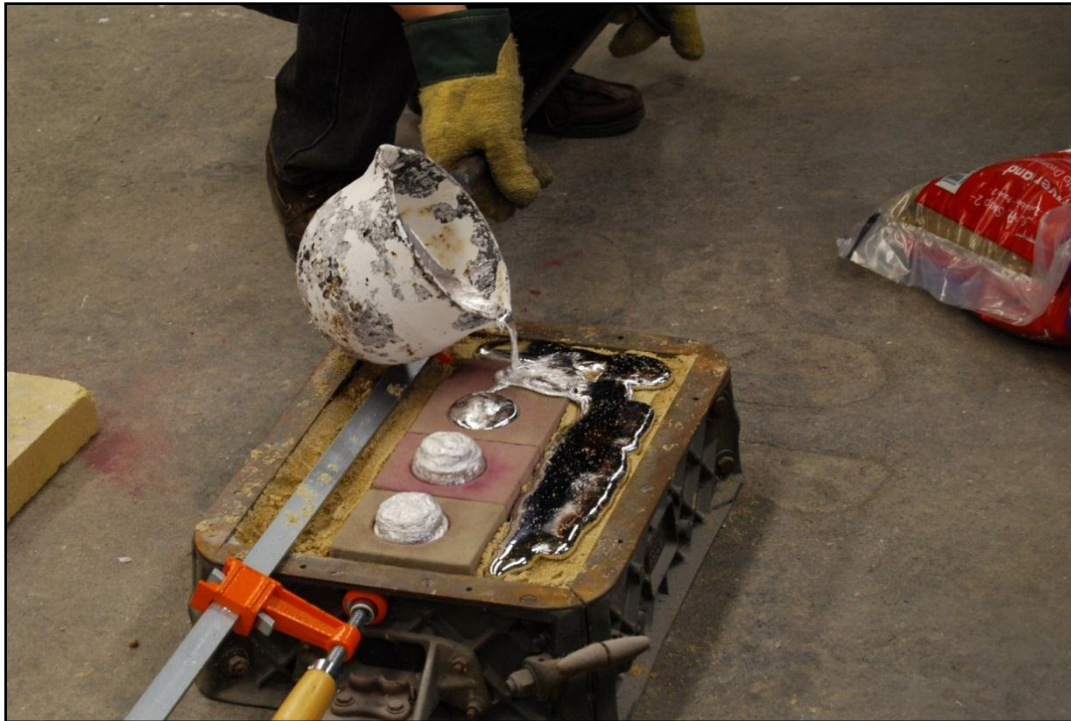
Figure 4-16: Aluminum metal pour using the three treated molds
