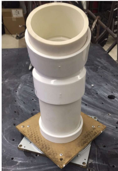
Figure 36 - Rotating PVC Pipe Assembly
