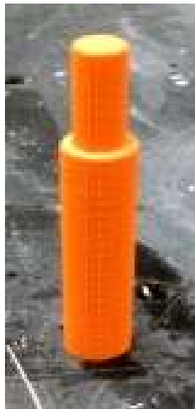
Figure 28 - 3D Printed Motor Alignment Tool
