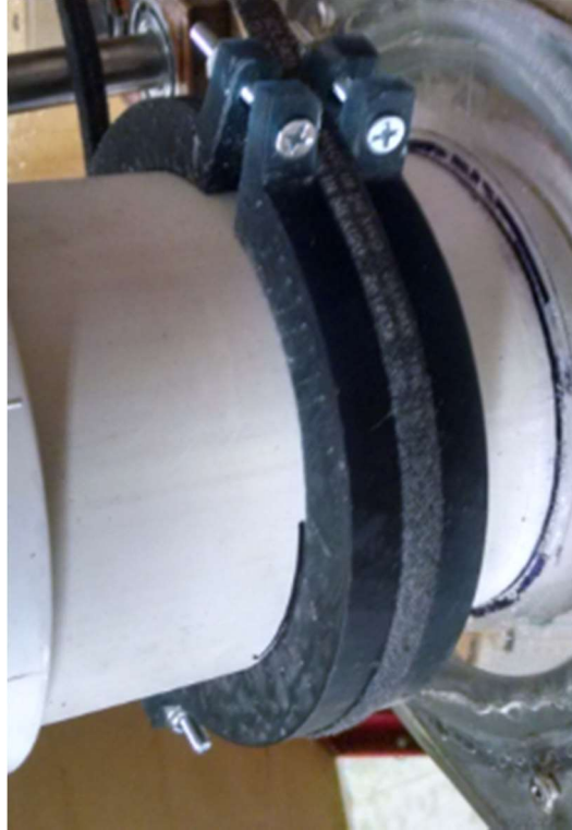
Figure 37 - 3D Printed Guide for Belt
