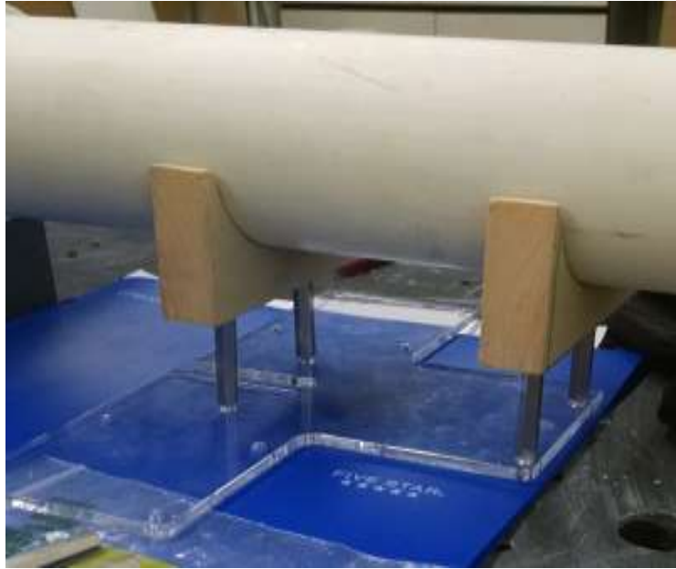
Figure 30 - Pine Wood Pipe Supports
