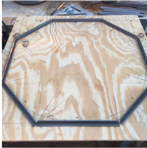
Figure 40 - Octagon Weld with Plywood Base
