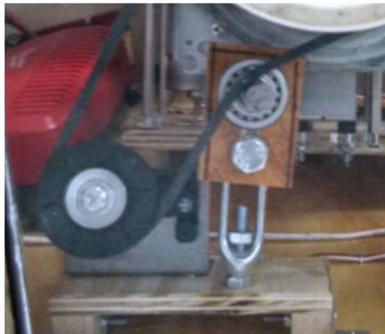
Figure 39 - Idler for Belt Tension
