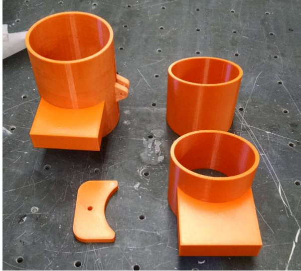
Figure 33 - 3D Printed Parts for Loader
