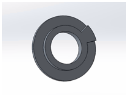
Figure 11: Key that fits over the central wing dowel and limits airfoil motion
