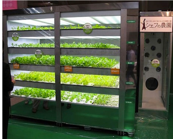
Figure 14 Climate-Controlled Lettuce Vending Machine [9]
