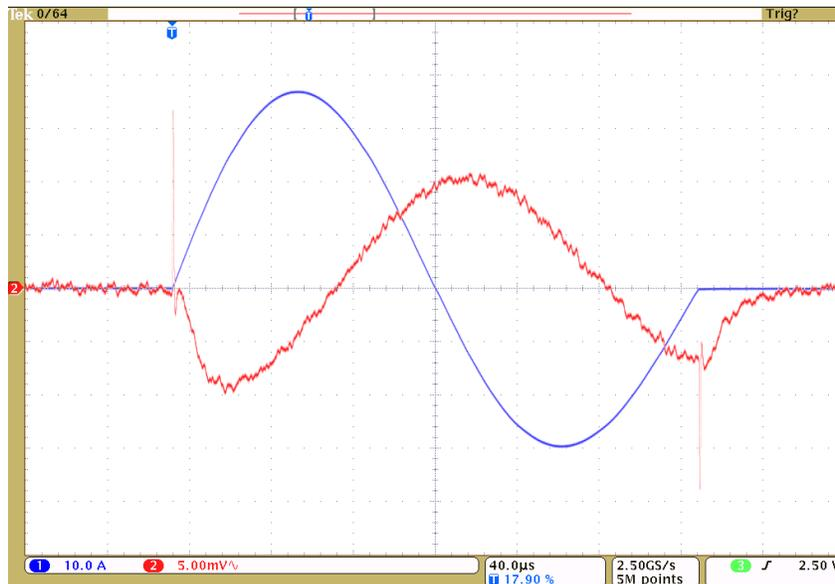
Figure 22: Measured induced electric field waveform at  $x=4.524\text{cm}$ ; the SNR at these measurement amplitudes was improved by averaging the waveform 64 times resulting in the waveform shown. CH1 (blue) is the coil current measured with a separate current probe in series with the coil, and CH2 (red) is the output voltage of the electric-field probe. The excitation frequency is 3.846kHz.
