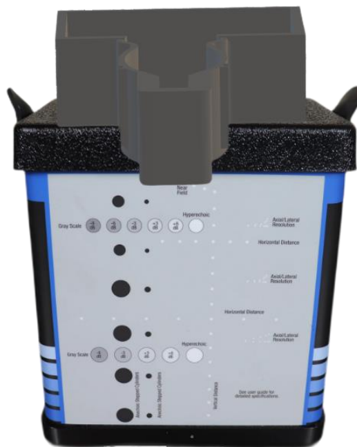
Figure 16 Representation of what the attachment (top) would look like placed on the CIRS Phantom (Bottom box) 11
