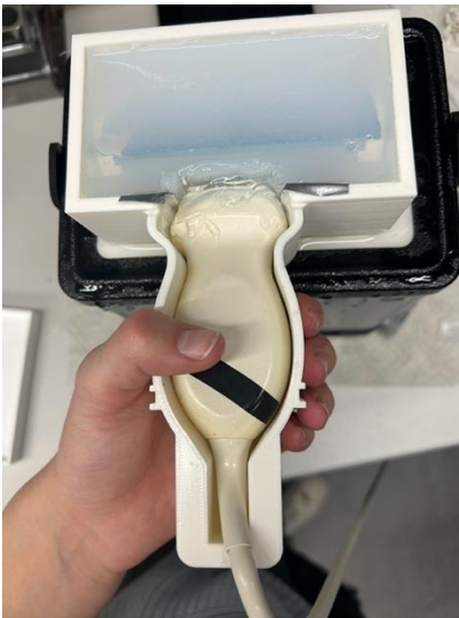
Figure 24 Cutout of gelatin to fit the ultrasound (above view)
