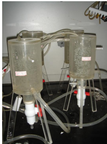
Figure 10 Up-Flow Aeration Bioreactors
