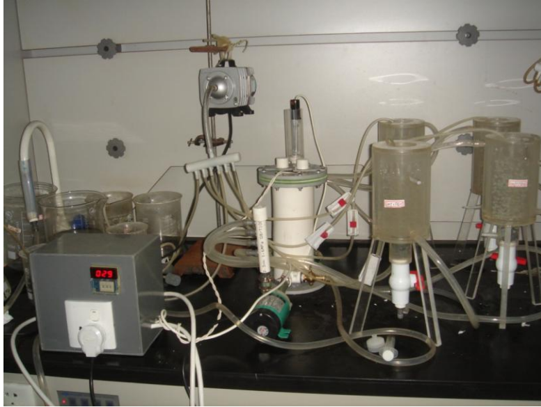
Figure 9 Set Up of Aeration System
