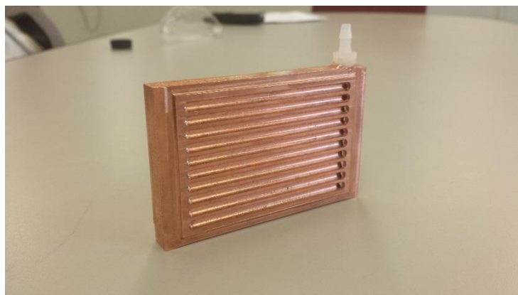
Figure 17: Epoxy sealed pipe adapter
