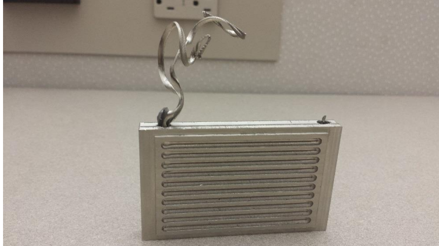
Figure 18: Nickel plate with broken drill bits
