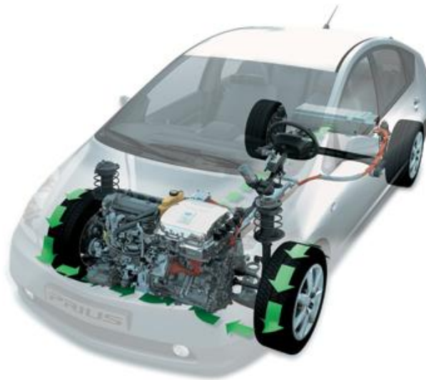
Figure 1-4 Prius Cut away showing both electric motor and gas engine.
