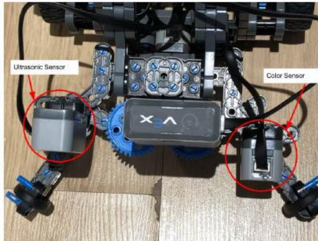
Overhead view of Ultrasonic and Color sensors
