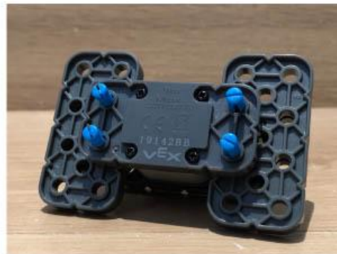
The back of the detached bumper sensor assembly
