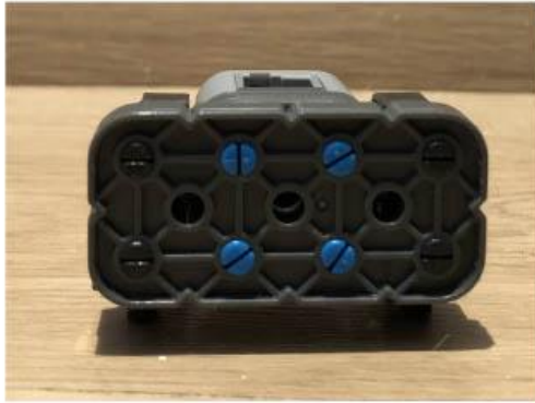
The back of the detached color sensor assembly
