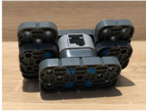
The front of the detached bumper sensor assembly
