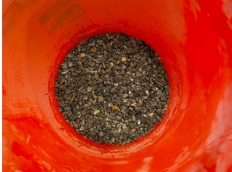
Figure 7: Image of gravel and half of water mix (before added cement)
