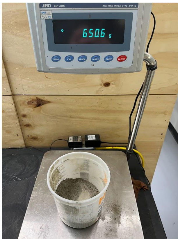
Figure 6: Image of Cement being weighed
