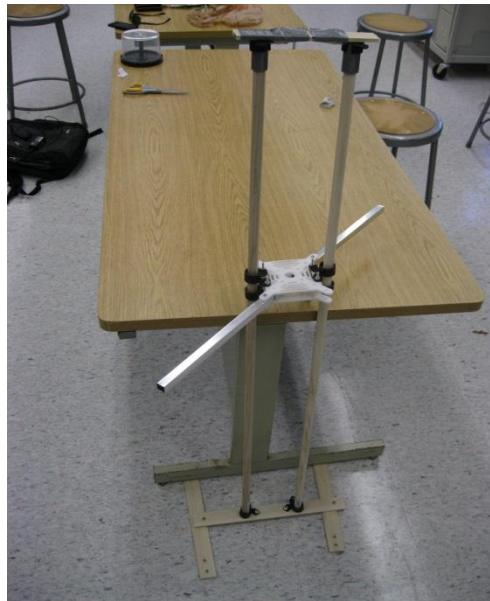
Figure 9-4: Vertical Thrust Test Stand
