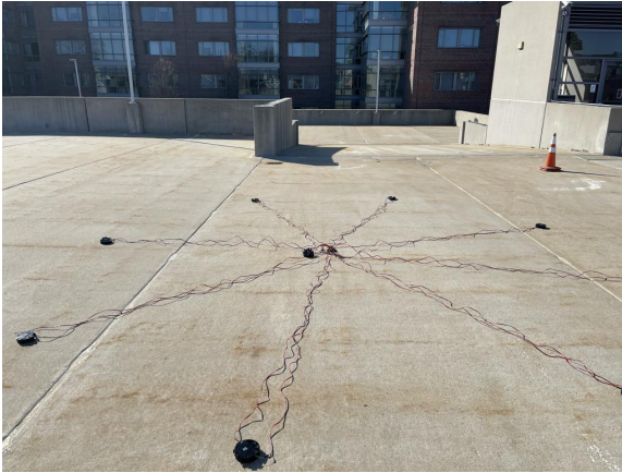
Figure 6: (Moreira et al. 2021) Old CMVS design set up for testing.
