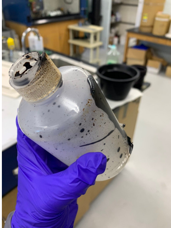
Figure 11. Overpressurized 250 mL HDPE bottle aftermath.
