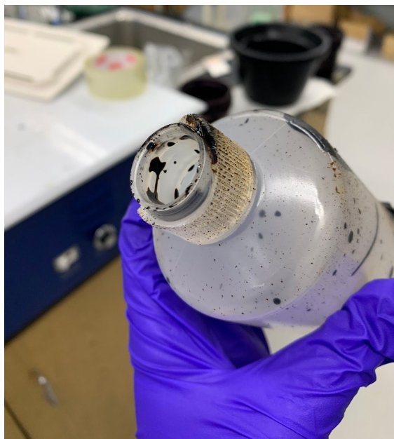
Figure 8. Overpressurized 250 mL HDPE bottle. Cap blown out.
