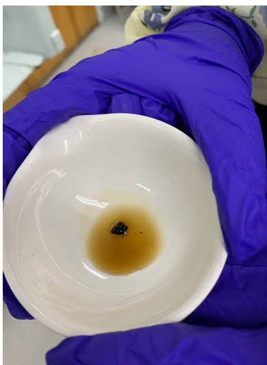
Figure 29. Resin dissolved in DMSO at 50 °C for 24 hours
