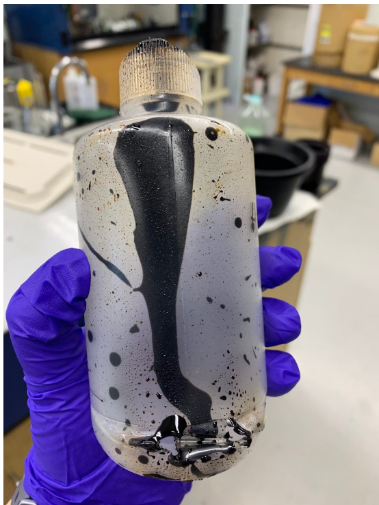
Figure 10. Overpressurized 250 mL HDPE bottle aftermath.
