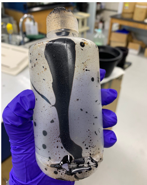
Figure 10. Overpressurized 250 mL HDPE bottle aftermath.
