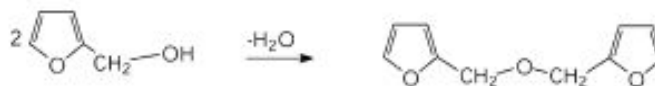
Figure 4. Condensation Reaction of Furfuryl Alcohol Resulting in the Formation of Dimethylene Ether Linkage (Bertarione et al.)
