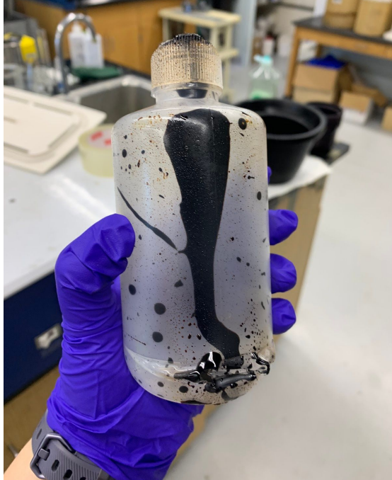
Figure 9. Overpressurized 250 mL HDPE bottle aftermath.
