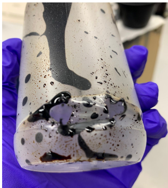
Figure 7. Overpressurized 250 mL HDPE bottle. Hole blown out at bottom.
