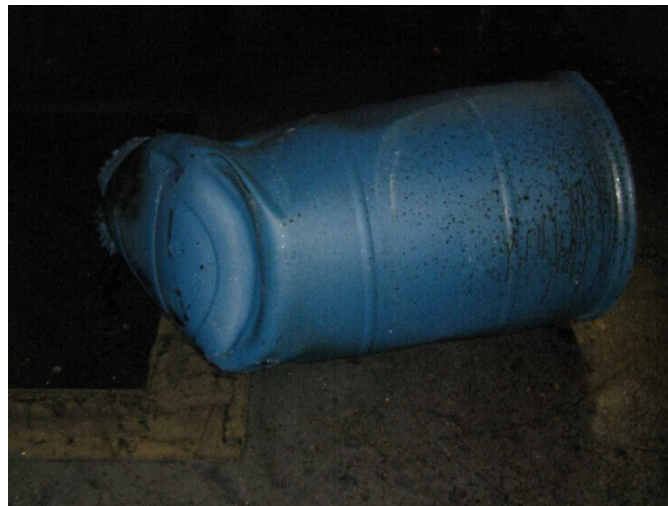
Figure 2. Overpressurized and overheated drum aftermath
