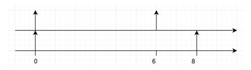
**Figure 1:** Example of simulation of a set of two tasks with respective periods  $p_1 = 6$  and  $p_2 = 8$
