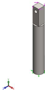
**Figure 91: Restraint and Load Surfaces for Main Shaft.**
