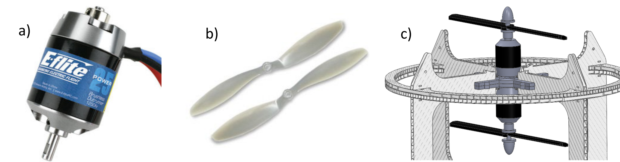
Figure 4 – a) Actual motors used in the IPASS, b) Actual propellers used in the IPASS c) CAD model showing the mounting of the propulsion system
