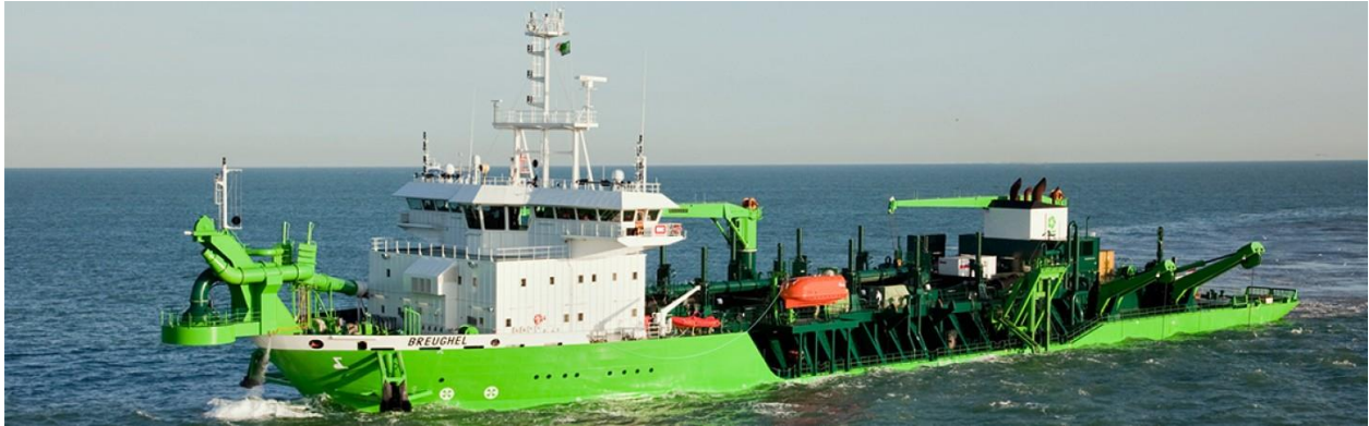
Figure 8: Brueghel Trailer Suction Hopper Dredge (Dredging International, 2014)
