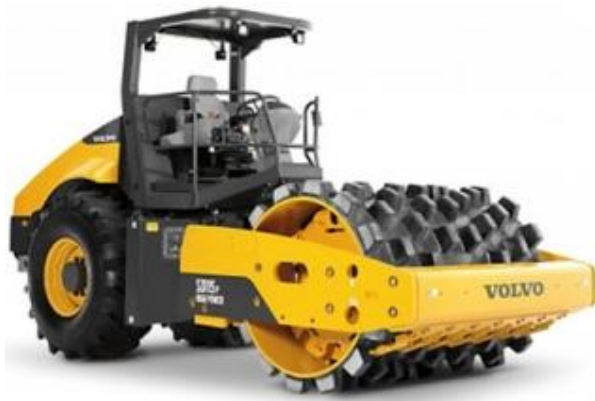
Figure 51: Sheepsfoot Roller (Sheepsfoot Roller, 2014)
