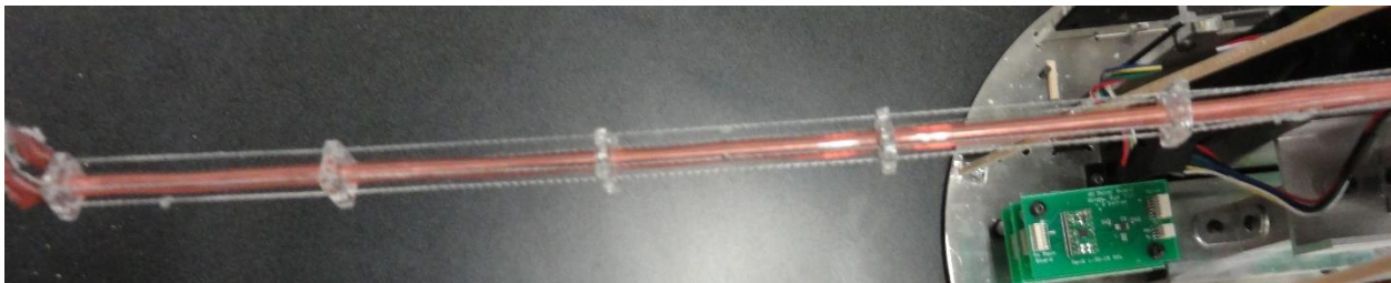
Figure 24: Picture of assembled wing without external shell components
