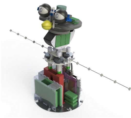
Figure 11: Solidworks rendering of entire robot without outer shell, showing internal layout and mechanisms
