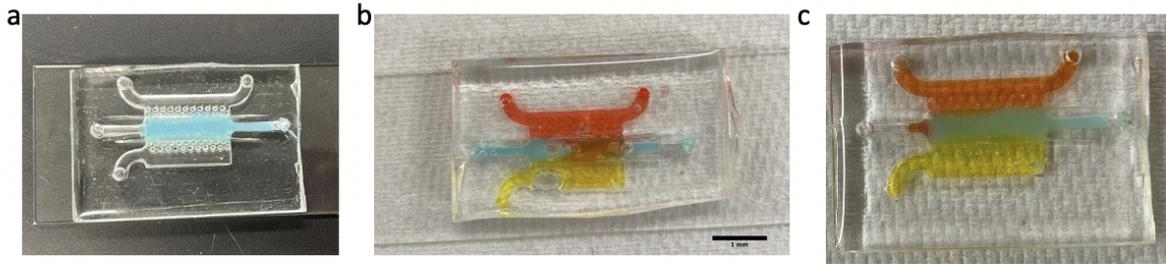
**Figure 16: Hydrogel retention and leakage test**
