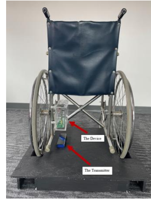
Figure K: Image of the system attached to the wheelchair and parked at the docking station.
