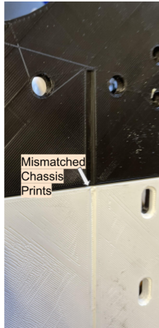
Figure 7-51: Misaligned Chassis Halves
