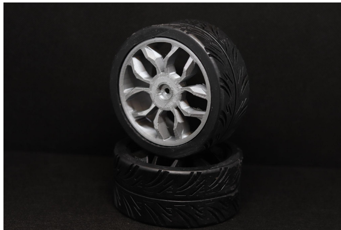
Figure 7-44: Final 3D Printed Wheel Assembly (PLA Interior and Flexible Resin Exterior)
