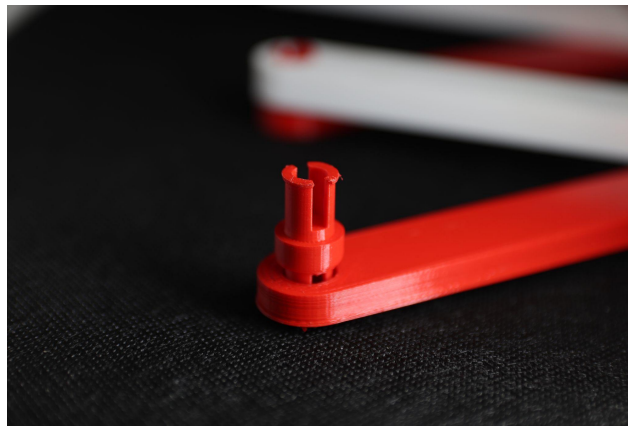
Figure 7-53: PLA printed fastener on scissor lift linkages
