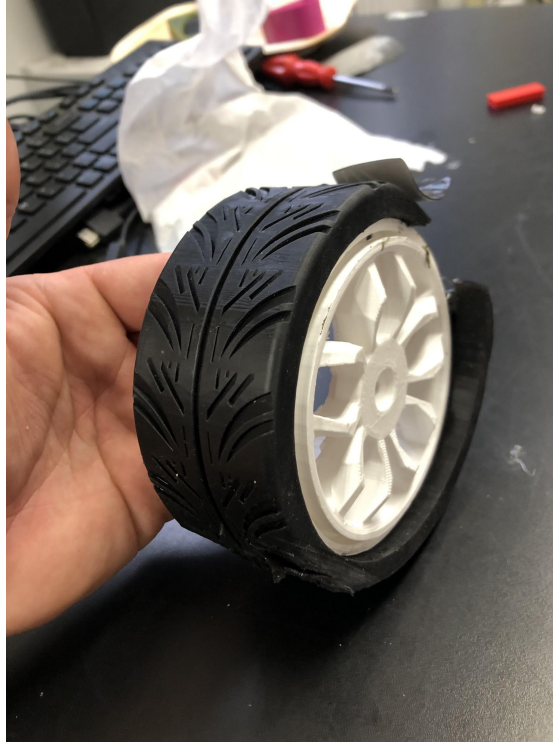
Figure 7-43: Failed Tire Resin Print with a Flat Spot
