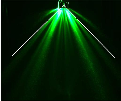
**Figure 8: Method Used to Measure the Spray Angle**
