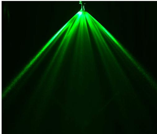
**Figure 9: Combined 500 Pictures of 65 Degree Nozzle with  $0.1365 \text{ m}^3 \text{ s}^{-1} \text{ Pa}^{-1/2}$  K-factor at a pressure of 1.38 bar (20 psi)**
