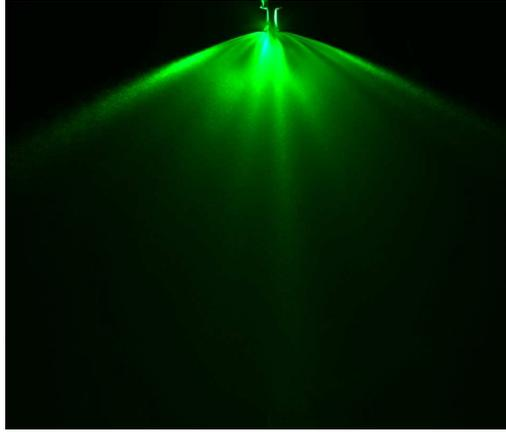
**Figure 10: Combined 500 pictures of 125 Degree Nozzle with  $0.2277 \text{ m}^3\text{s}^{-1}\text{Pa}^{-1/2}$  K-factor at a pressure of 1.38 bar (20 psi)**
