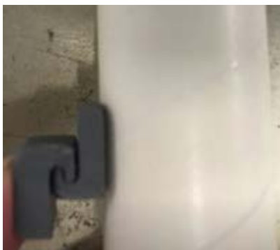
Figure 17. Image of 3D-printed booster hooks and booster tube.
