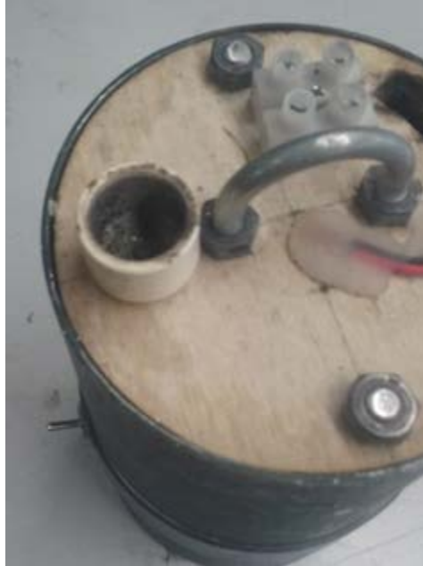
Figure 7. Black Powder separation system charge well.
