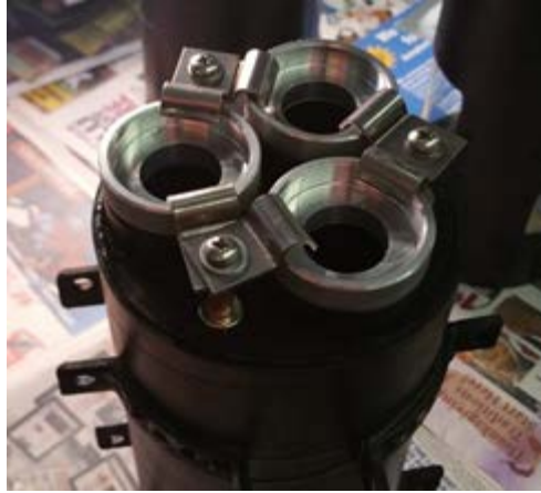
Figure 12. Image of the motor retention system over empty motor mount tubes.
