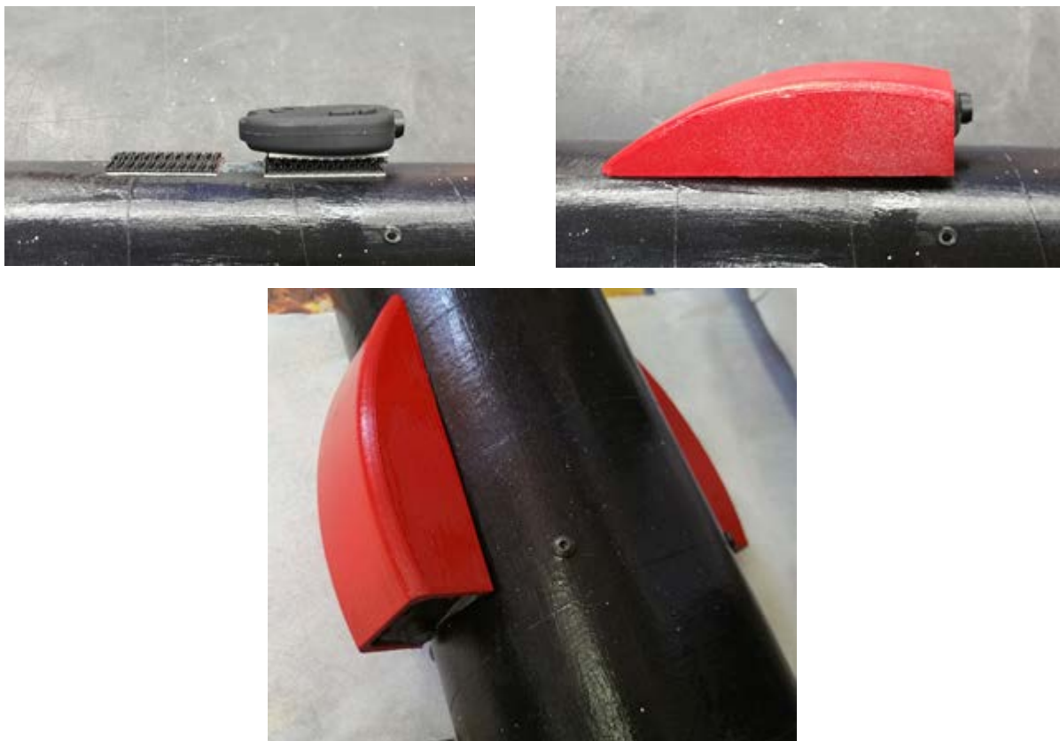
Figure 21. Images of the side camera mounted to the airframe. The red fairing can be independently removed from the rocket to access the camera.
