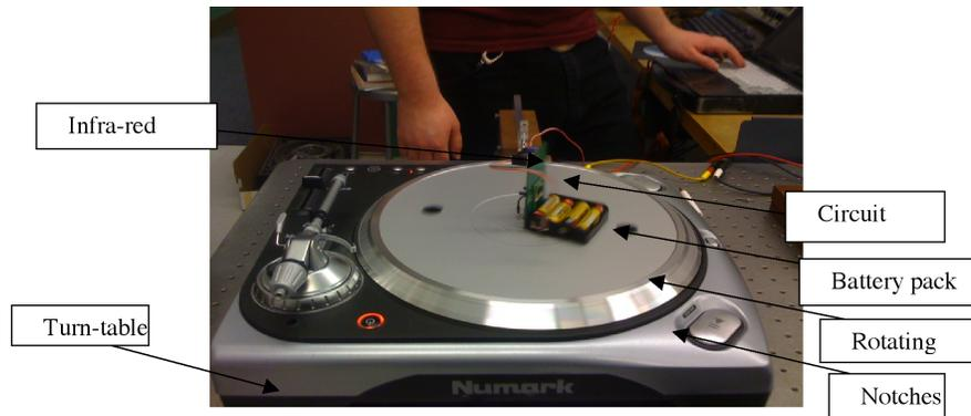
Figure 3.25: Turn-table set-up
