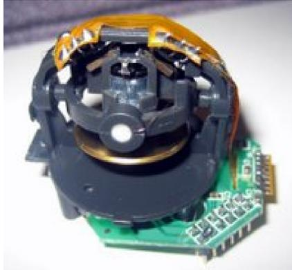
Figure 3.1: Low quality mechanical gyro from X-UFO.
