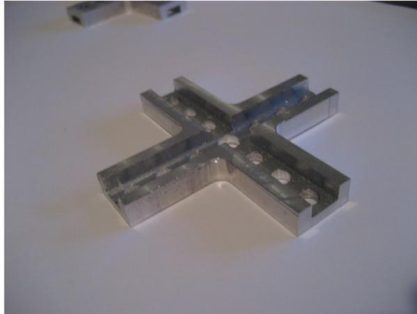
Figure 3.14: One half of the post manufacture central hub.
