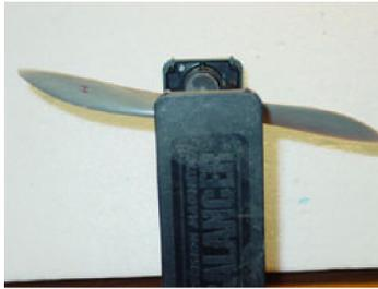
Figure 3.24: Satisfactory orientation of a balanced propeller.
