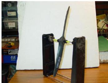
Figure 3.21: An unbalanced propeller.
