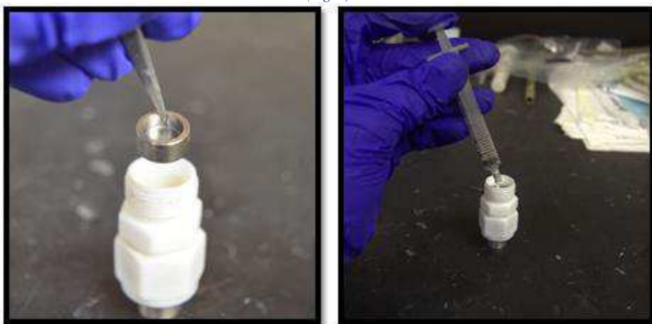
Figure 3: Swagelok PTFE union connected to fitting holding anode current collector (left). Addition of compression spring (right).
