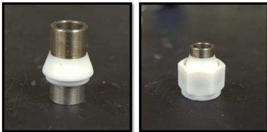
Figure 2: Ferrule orientation on anode current collector (left) in Swagelok PTFE fitting (right).
