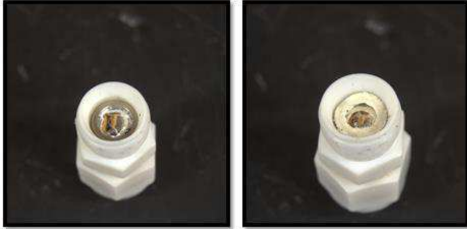
Figure 5: View of liquid gallium in crucible (left). Teflon gasket above anode crucible (right).
