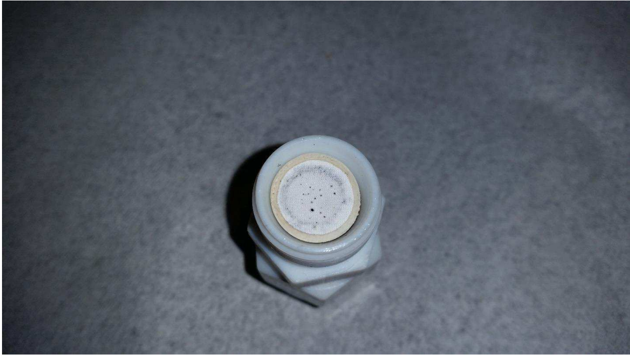
Figure 4-30: Through-plane gallium leakage to the anode, short circuiting the cell.
