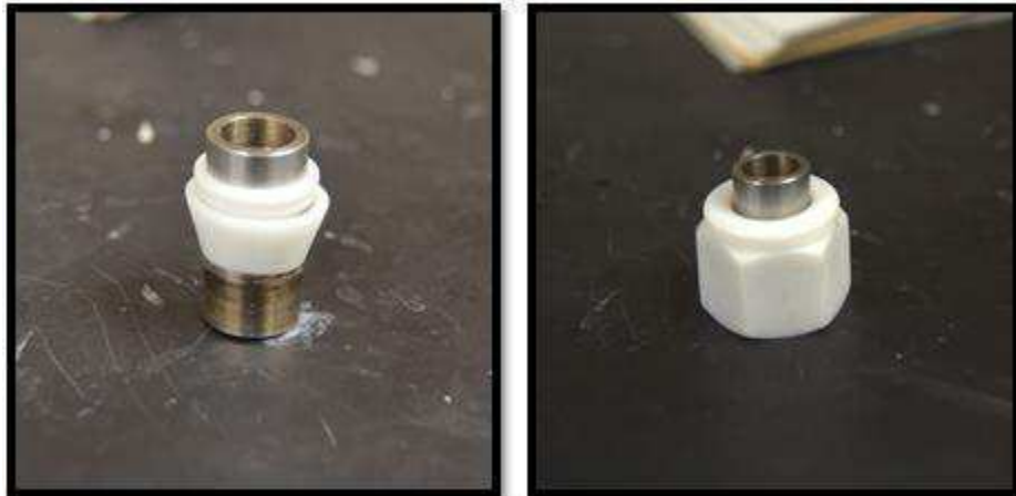
Figure 7: Ferrule orientation on air cathode current collector (left) with Swagelok fitting added (right).
