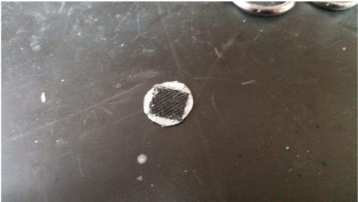
Figure 4-33: A zirconia separator covered with a GDL after a high temperature test
