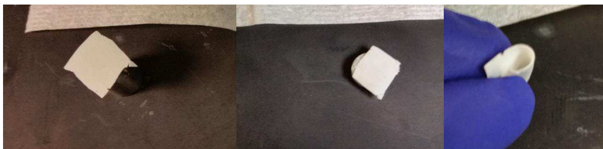
Figure 4-32: Left: An unsoaked zirconia cloth separator. Middle: A KOH wetted zirconia cloth separator. Right: A dried zirconia cloth separator, previously KOH wetted.
