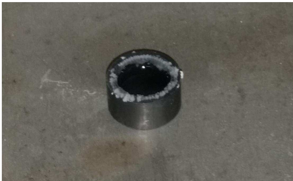
Figure 4-31: KOH/NaOH eutectic heated and monitored for carbonation.
