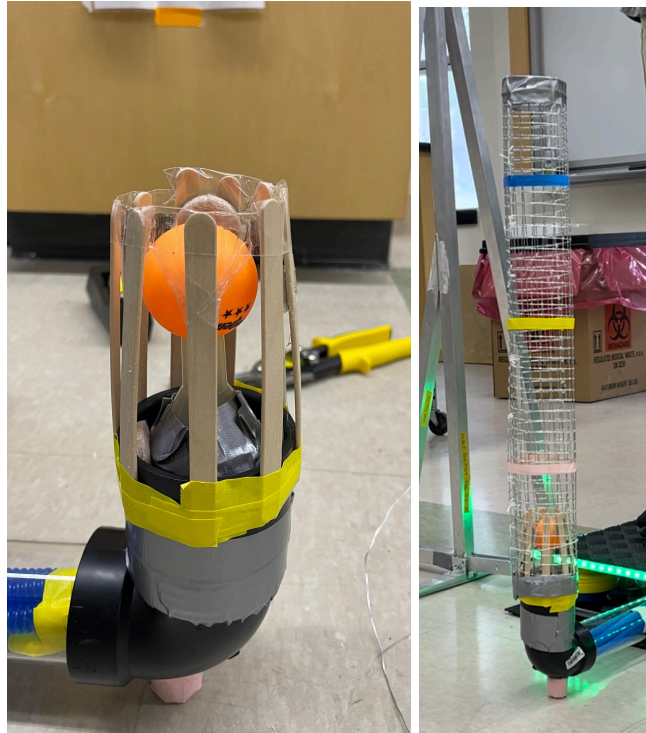
Figure 18. Ball pump mechanism with the angled wooden sticks (left) and wire mesh (right)
