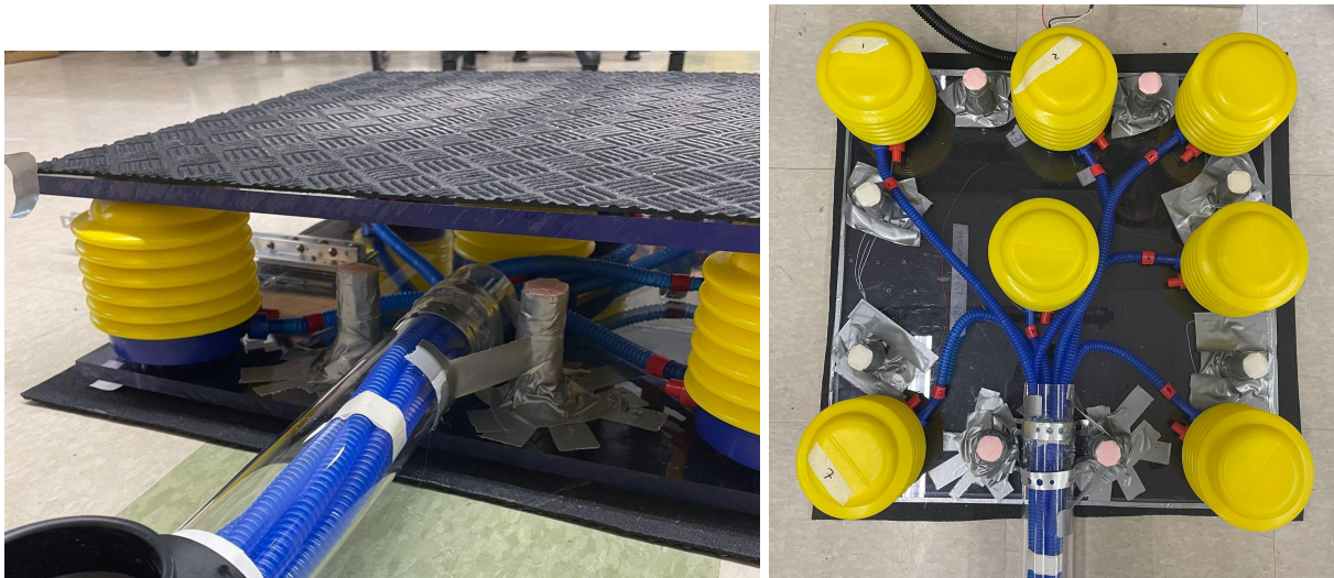
Figure 15. Final version of the pump mechanism with the addition of stoppers on all sides of the jump platform
