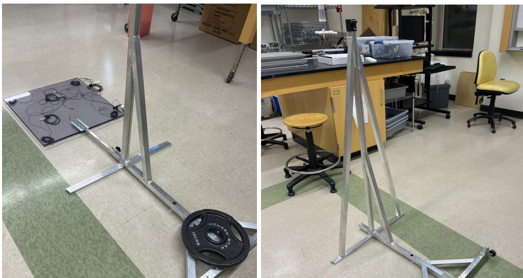
Figure 22. Initial assembly of the vertical jump stand (left) and the stand with extra supports (right)
