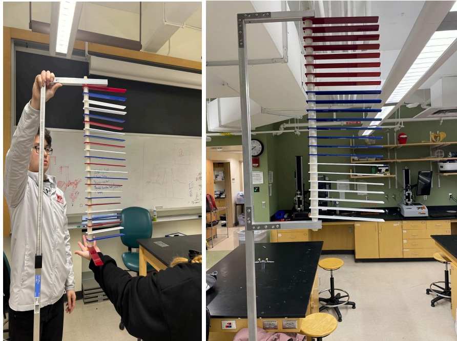
Figure 25. Rungs before (left) and after (right) initial testing
