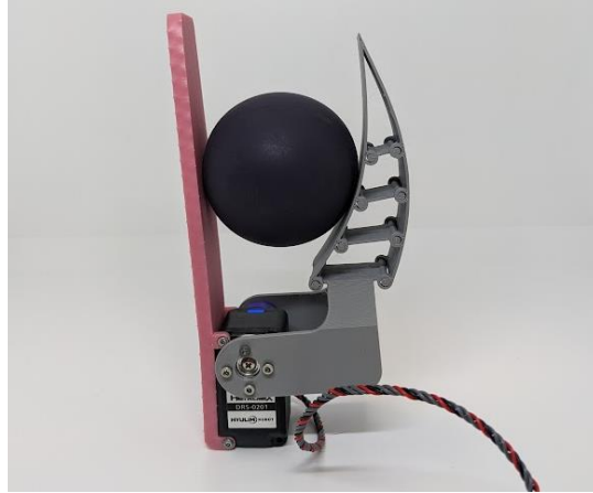
Figure 25: Hybrid two-finger pinch gripper holding a rubber ball
