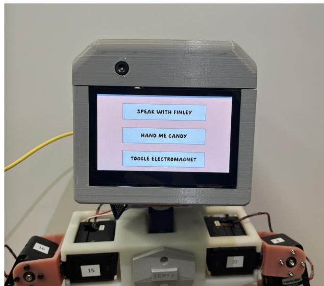
Figure 47: PyGame control screen with microphone
