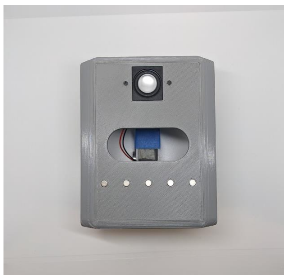
Figure 30: Magnet and speaker included on head lid
