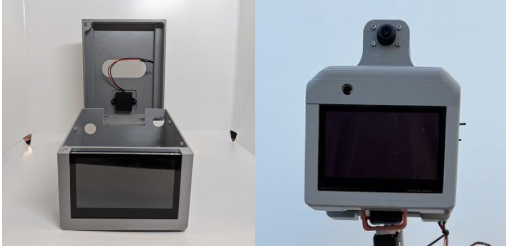
Figure 31: Finley's head with the onboard sensors attached as well as the camera attached on top of the lid using magnets
