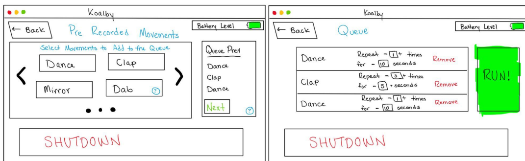
Figure 13.1: First UI LoFi Prototype Mockup of Pre-Recorded Movements (left) and Queue Editing Page (right)
