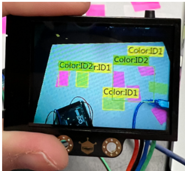
Figure 9.17: Huskylens trained on two colors
