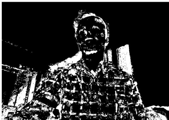
**Figure 7: OpenCV Performing Background Subtracting and Showing Contour Highlights**
