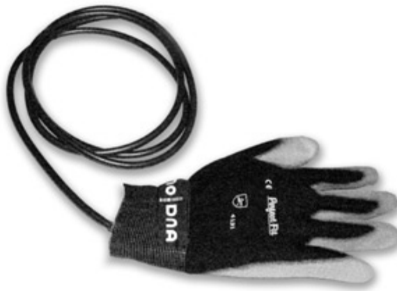
Figure 17: X-IST data glove using fiber optic bend sensors 14
