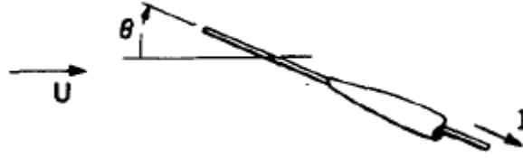
Figure 13: Probe Angle of Attack in a Plasma with Drift Velocity U [22]
