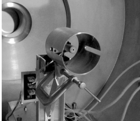
Figure 21: Anode Configuration Allowing Langmuir Probe Traverses [10]
