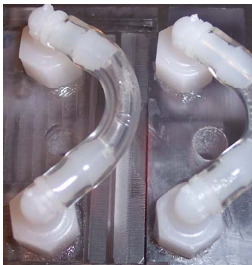
Figure 49: Example of Luers Checked During Leakage Study
