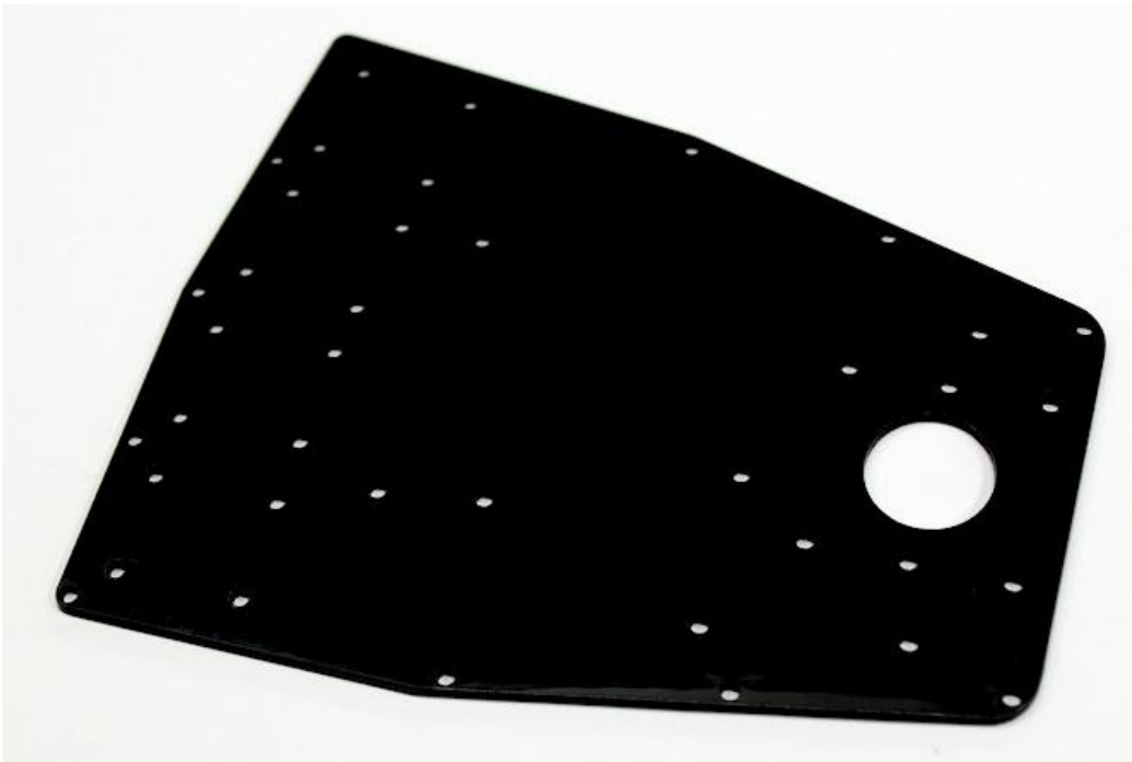
Figure 54 Laser Cut Delrin Chassis Plate Standing In for Carbon Fiber
