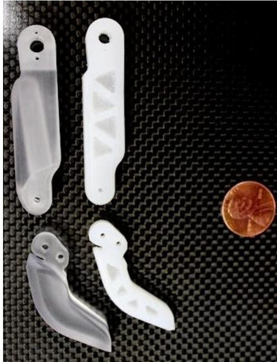
Figure 62 Final Polycarbonate Finger Parts Next to Earlier Finger Parts
