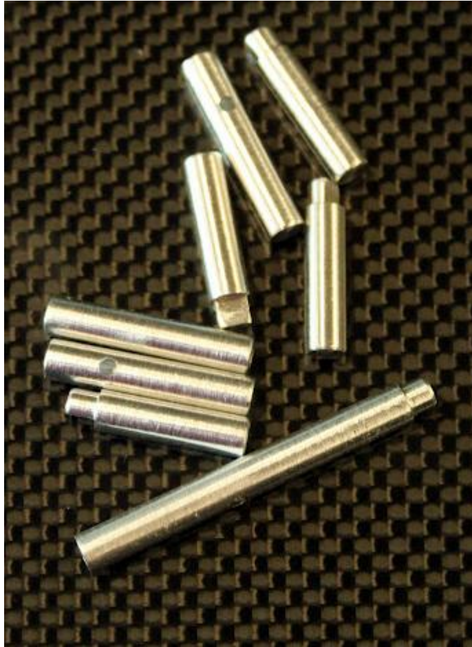
Figure 55 7075 Aluminum Final Gearbox Shafts
