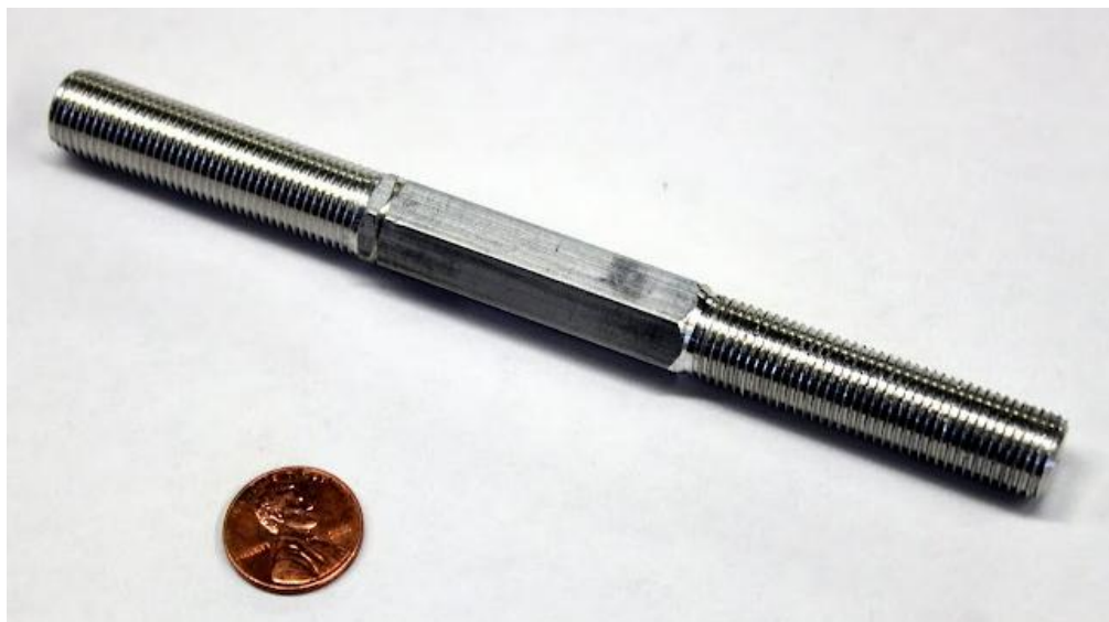
Figure 52 Aluminum 1/2-20 Stud Turnbuckle Awaiting Modification
