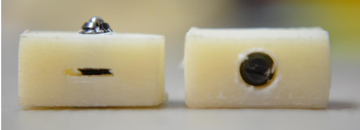
Figure 5.1.19: Ball Plunger Blocks with Ball Plungers Installed
