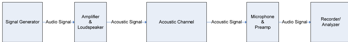
Figure 2. Loudspeaker testing setup.
