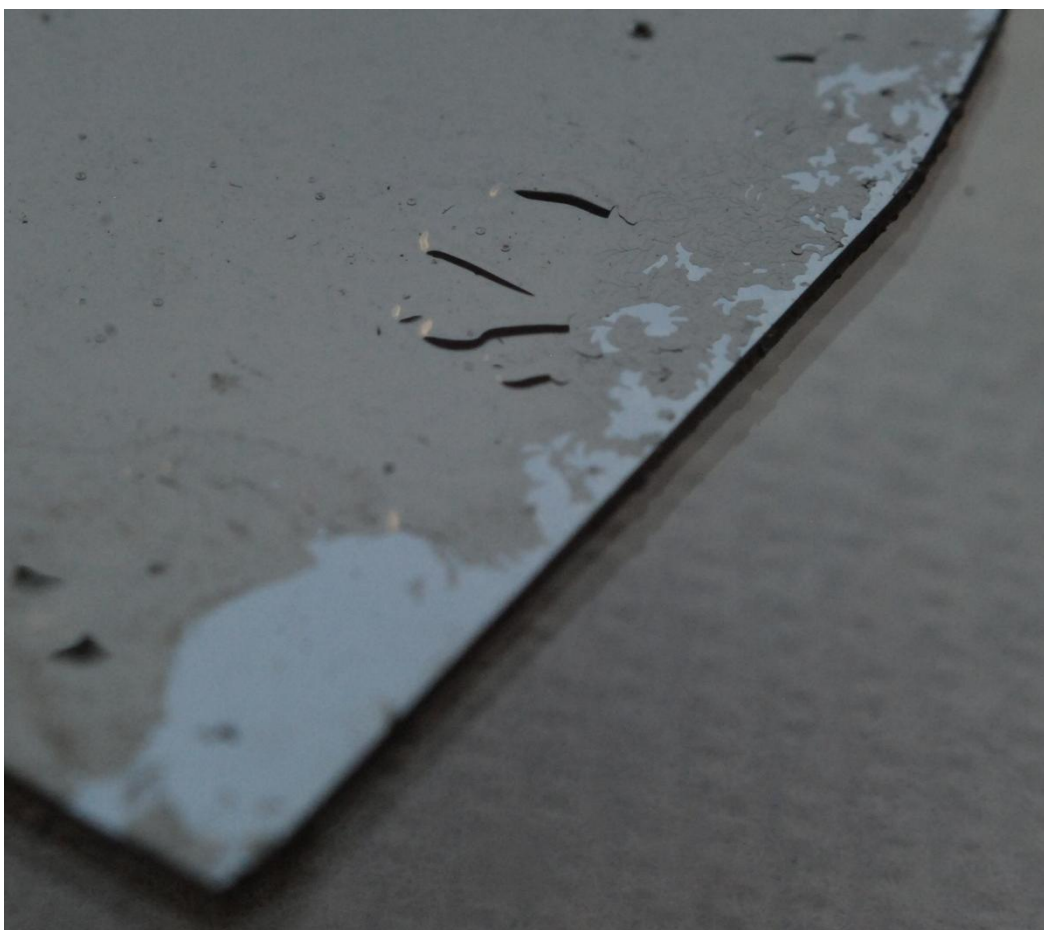
Figure 4.2.1.1: Photograph of cracking of carbon film.
