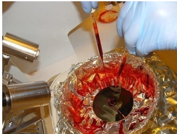
Figure E.11: Spin Coating Photoresist Application Technique The spin coater is activated by hitting the “START” button on the control consol. The spin coater will follow the predetermined and entered procedure and will automatically stop. After the spin coater has stopped and the applicator head has risen, remove the vacuum supply to the spin coater.
