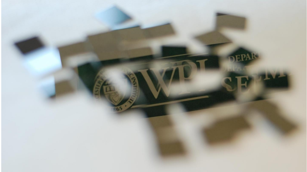
Figure 4.2.1.7: Photograph highlighting the reflective properties of properly fabricated carbon films.
