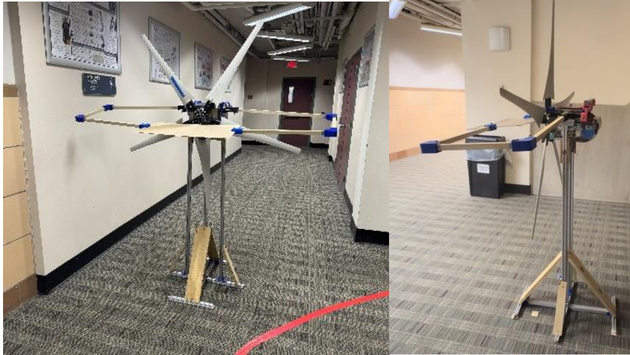
a. b. Figure 14: Base Leg Supports a. Back View and b. Side view
