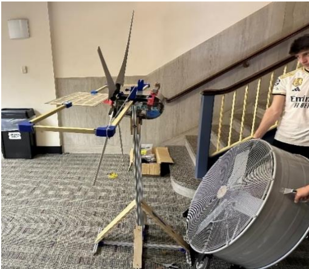
Figure 25: Tilting Mechanism Testing
