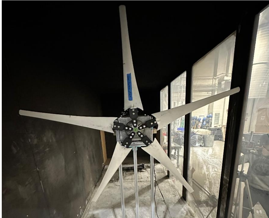
Figure 10: Turbine Hub, Rotor, and Blades
