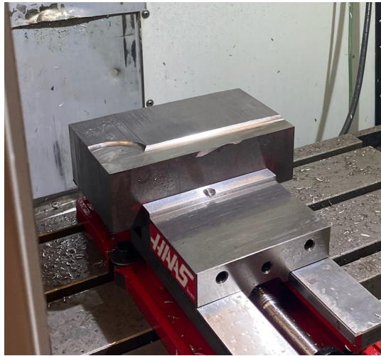
Figure 33: Facing Pass Where Machine Crashed
