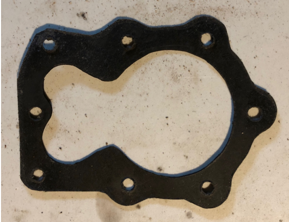
Figure 10: Custom Made Engine Head Seal Figure
