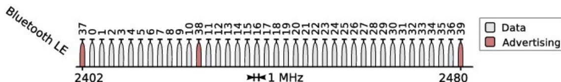
Figure 2.8: Bluetooth LE Channel Map. LE devices make use of 40 Channels, each 1 MHz apart, of which 37 are used to exchange data while the 3 advertising channels are used during the pairing process. [6]
