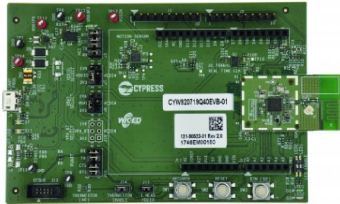
Figure 3.2: Overview of the EVB housing the CYW20719 Bluetooth IC used in this project [7] The EVB can be connected to a host computer using a micro-USB port shown on the left side. The built-in antenna is located on the daughter board on the right side
