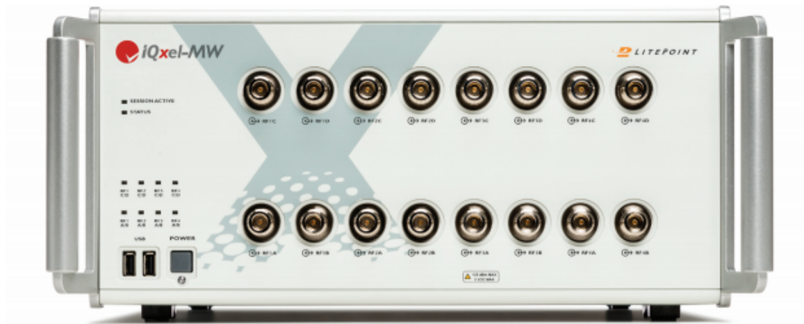
Figure 4.1: The Litepoint IQxel-M16W Used in the First Build of the Promiscuous Packet Capture System [8]. The ten status lights to the left indicate the on-off state of device, whether a session is active, and the status of each of the 8 modules. Each module consist of two ports that can be configured as an input or an output and monitored separately.
