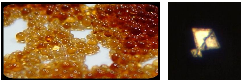
Figure 3. Left: A photograph of acid Amberlite ion exchange resin showing the polystyrene beads. The surfaces of these beads contain sulfonic acid functionalities in the form of sodium salt. Right: Single crystals of POSS-CN viewed under crossed-polarizers.
