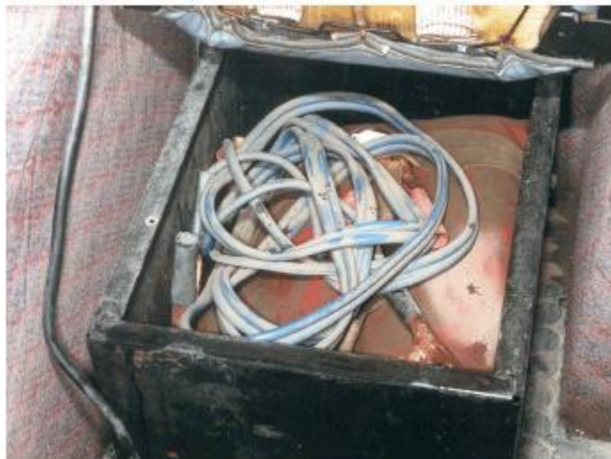
Figure 13: PFD with cables on top of it on Lady Duck. (Source: Transportation Safety Board of Canada, 2004, p. 40)
