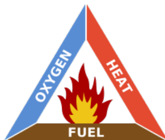
Figure 34 The Fire Triangle. As seen above, it is made up of three legs, oxygen, heat, and fuel. To have a fire, all components must be present. If one component is taken out during a fire, the result is extinguishment (CabelSystems, 2007).
