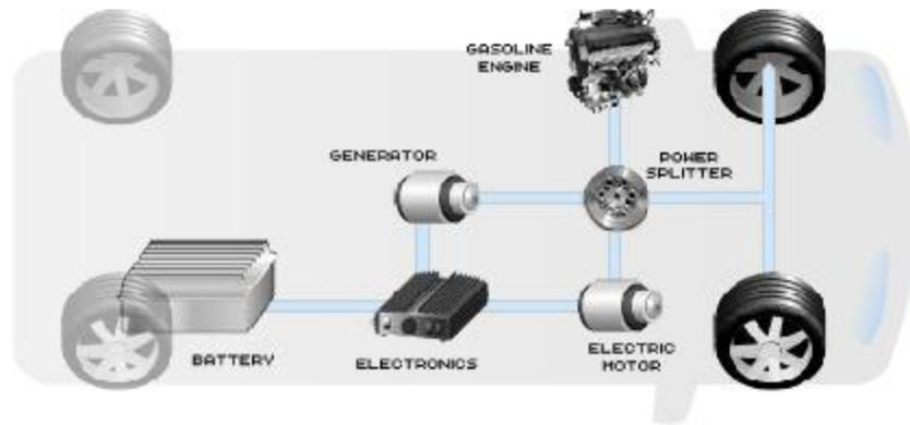
Figure 15 - Combination Drivetrain<sup>33</sup>
