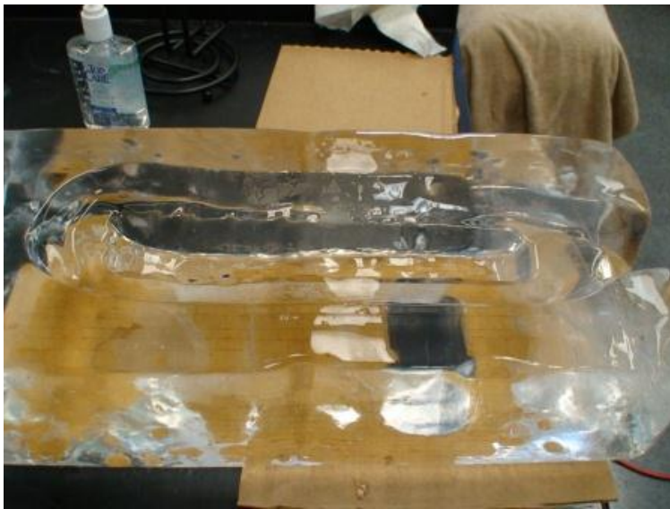
Figure A.9: Example of Oil Over Flow from Channel: Side View
