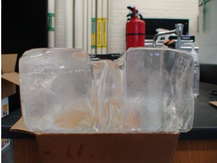
Figure A.8: Example of Oil Over Flow from Channel: Side View
