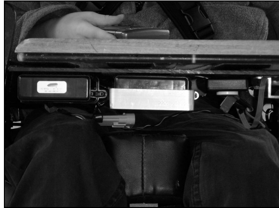
Close-up of sensing device mounted under Subject 3's lap tray. The actual device setup used in training was the unshielded sensor.
