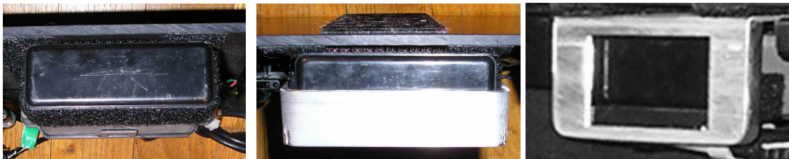
Figure 5: ROSS unshielded sensor (left), ROSS sensor with metal shield across bottom half (center), ROSS sensor with metal perimeter shield (right)
