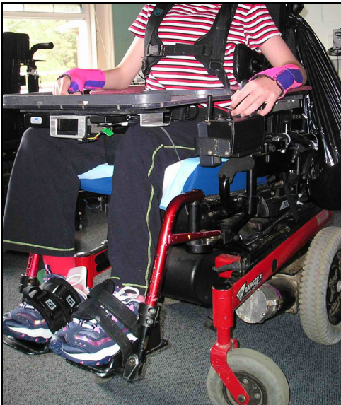
Isometric view showing Subject 1's joystick setup on her left and the sensing device mounted underneath her lap tray.
