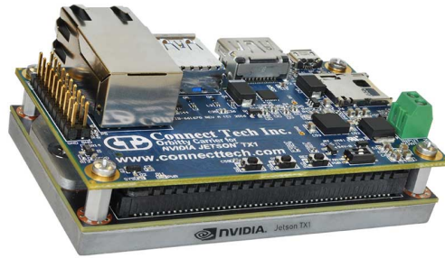
FIGURE 4.2: Jetson in Orbitty Carrier [20]
