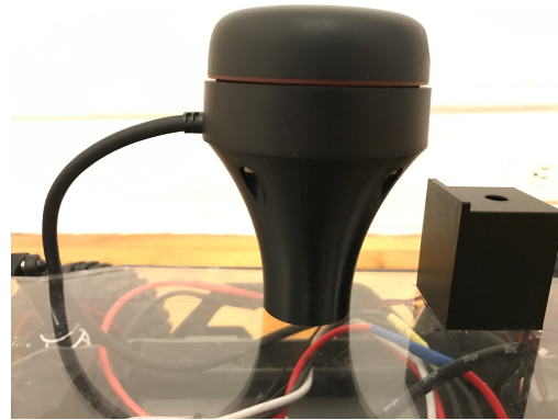
(B) 3D Printed Lidar Mount
