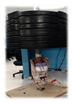
Figure 23 Socket under Weights for Testing
